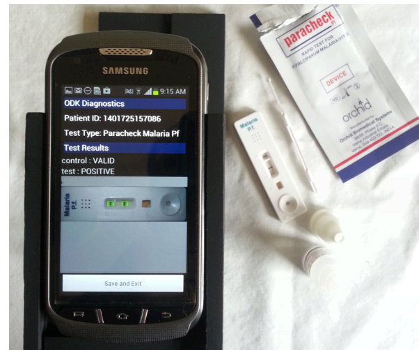
Figure 3: The mobile system's user interface, showing a processed diagnostic test for malaria with a positive result.
