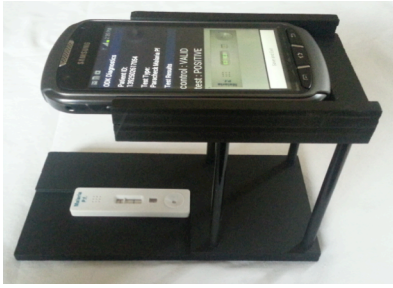
Figure 4: A simple plastic stand holds the mobile device in a convenient position above the diagnostic test.
